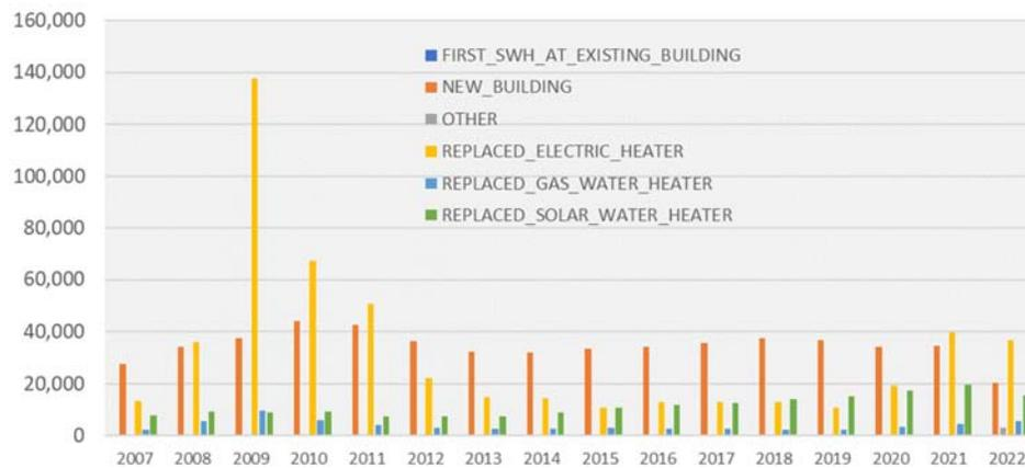
We estimate that more than 121,000 SWH and ASHP systems will be installed and create certificates in 2022 which is a 22% increase on 2021 levels. The most important driver for the increase has been policy support measures such as building regulations and energy efficiency schemes.
