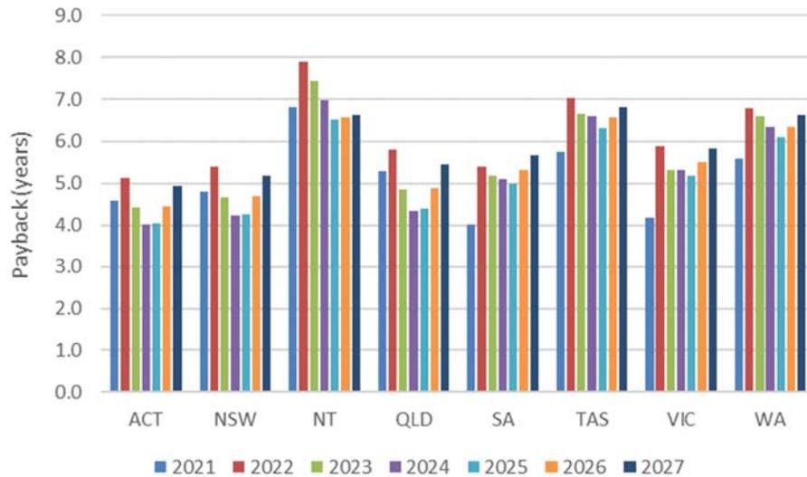
**Figure 3.6 Simple Payback (real) for typical Commercial PV system (20kW)**
