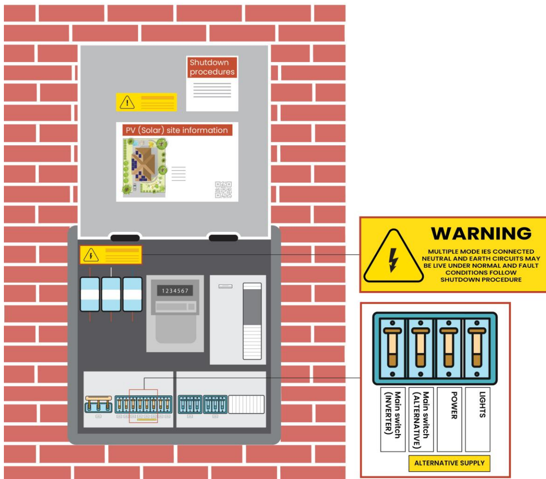
Figure 2: Example of critical labels located on the switchboard and the inside of the meter box cover
