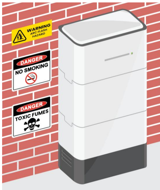
Figure 3: Example of labels mounted adjacent to the solar battery
