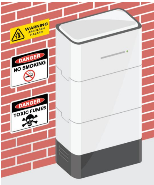
Figure 3: Example of labels mounted adjacent to the solar battery
