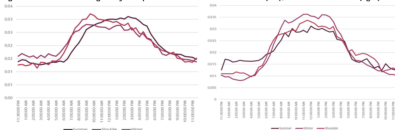
Figure 4: Normalised average daily load profiles for commercial customers (left), industrial customers (right).
