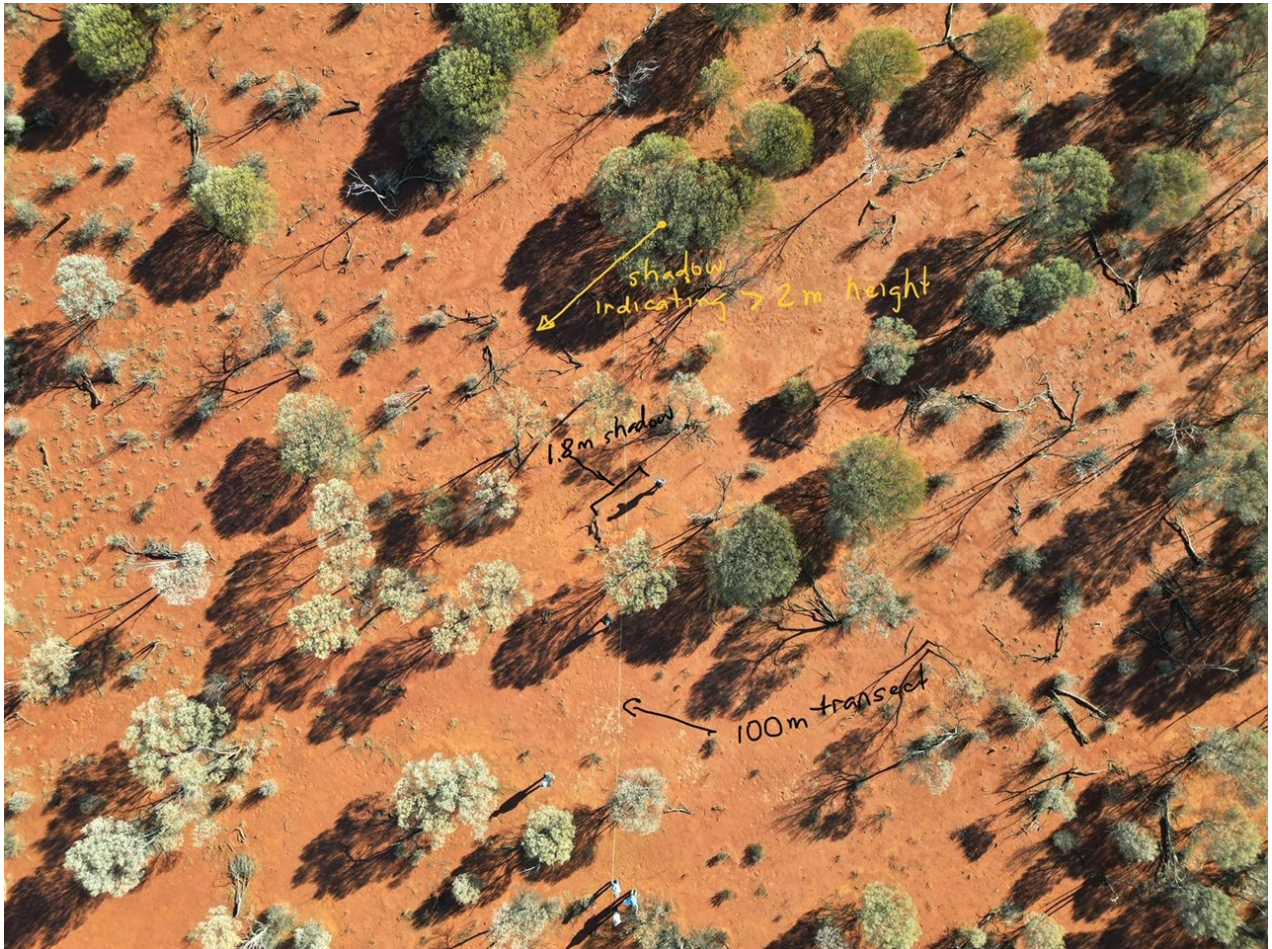
Figure 2: Orthogonal photograph (20 m above the ground) of a section of a 100 m transect laid out at a "point of interest" in Western Australia. Audit teams measured heights and canopy dimensions from the ground, but these can also be estimated from this aerial photograph (e.g., using the shadow cast by a person of known height)
