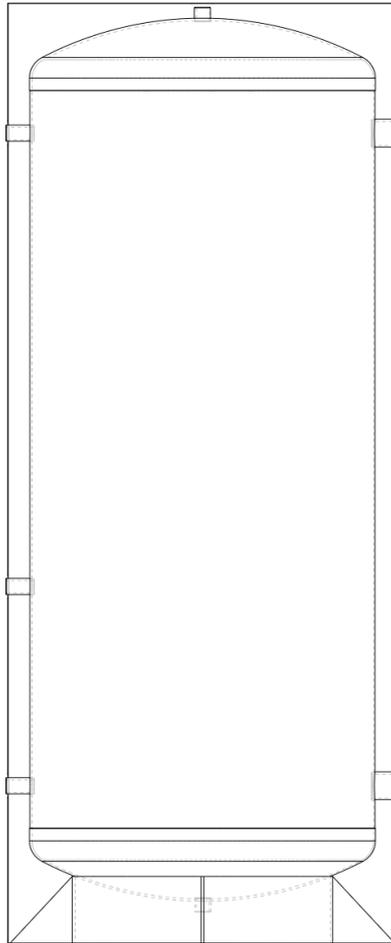
**Figure A1.** Large hot water tank resting on a ring that supports the tank on the ground. The inside of the supporting ring contains air, which substitutes for the insulation on the tank underside.
