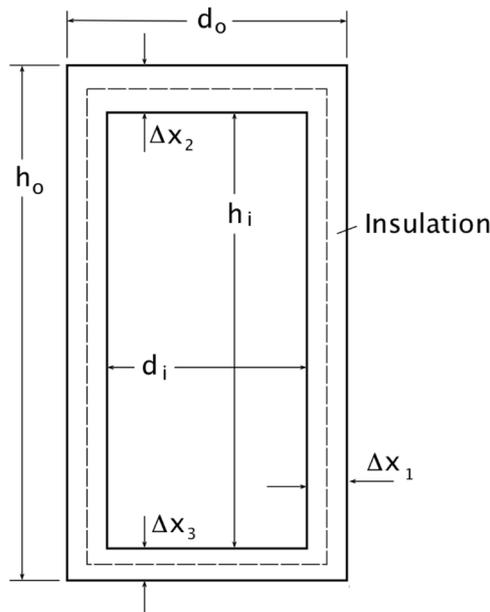
Figure 1. Cross sectional view through an idealised cylindrical tank of inner diameter  $d_i$  and height  $h_i$  covered with insulation of thickness  $\Delta x$ .
