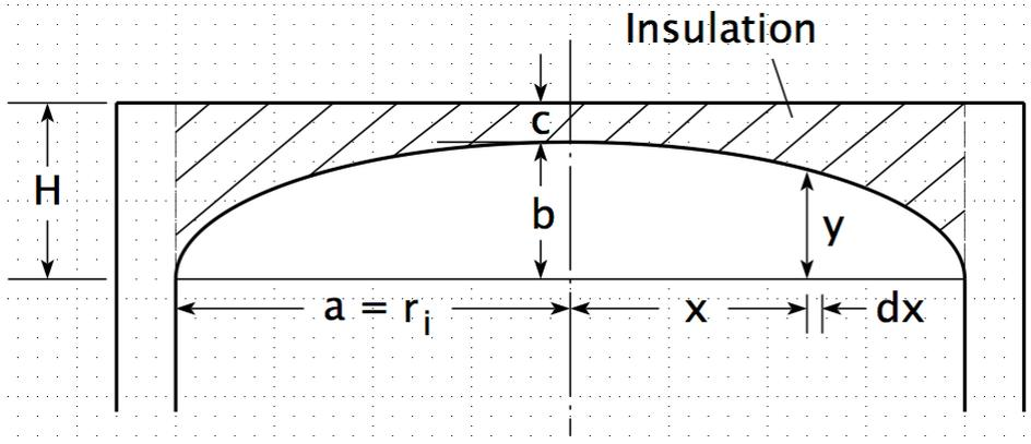
**Figure A2.** Schematic diagram of the top section of a hot water tank with an ellipsoidal dome, where  $a$  and  $b$  are one-half of the ellipse's major and minor axes respectively. The average insulation thickness above the tank dome can be determined by calculating the volume of the insulation above the dome and dividing the volume by the circular area below the dome.
